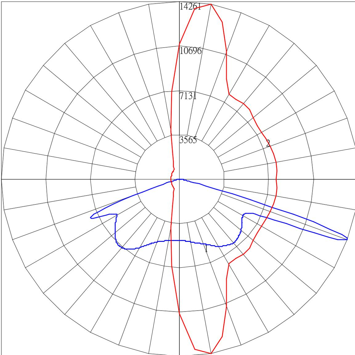
Maximum Candela = 14261.041 Located At Horizontal Angle = 80, Vertical Angle = 70
