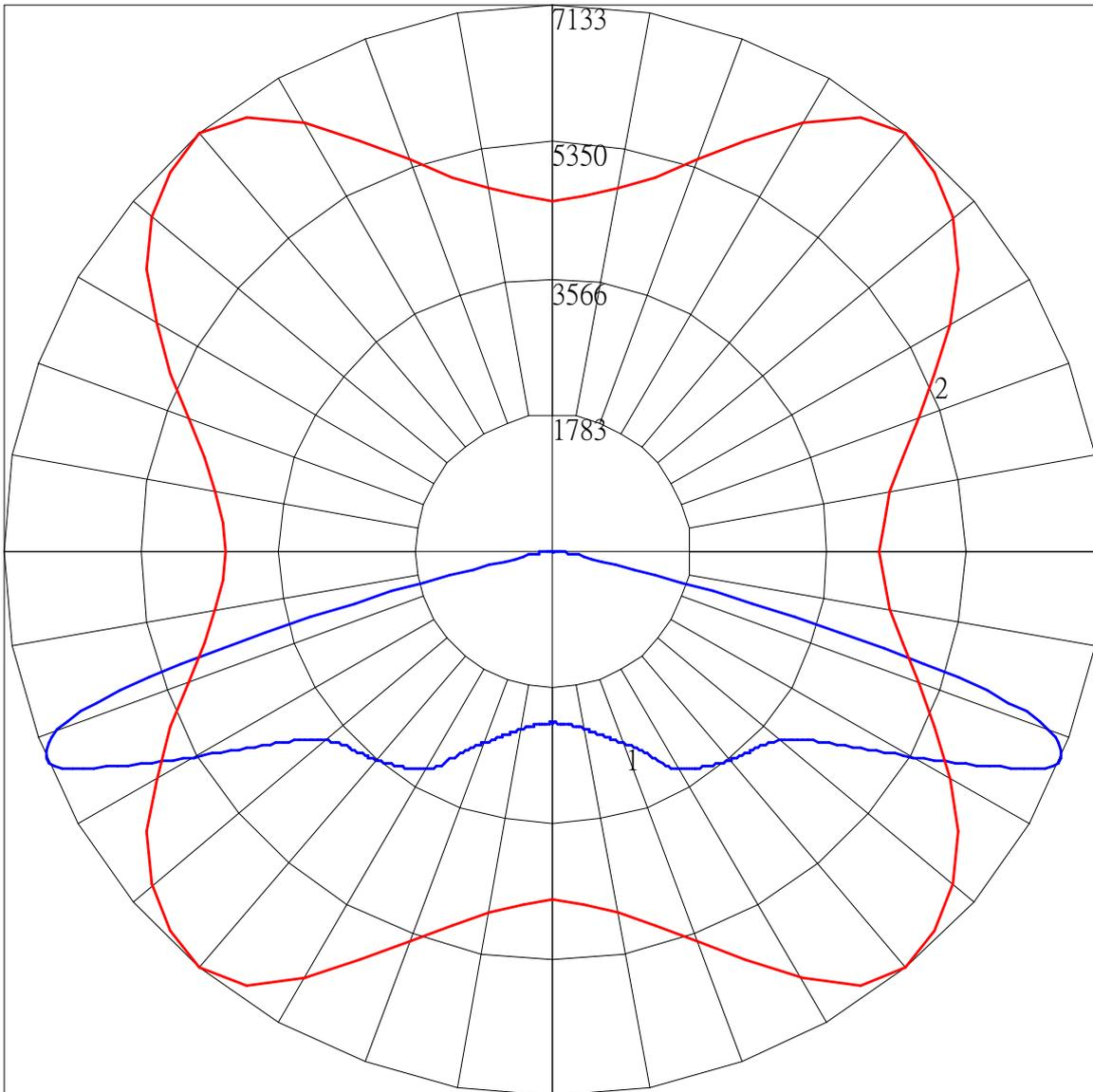
Maximum Candela = 7132.693 Located At Horizontal Angle = 50, Vertical Angle = 67.5
