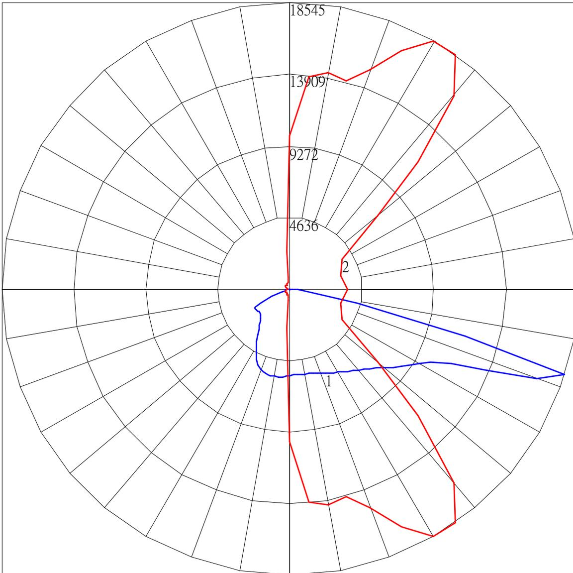
Maximum Candela = 18544.876 Located At Horizontal Angle = 305, Vertical Angle = 72.5
