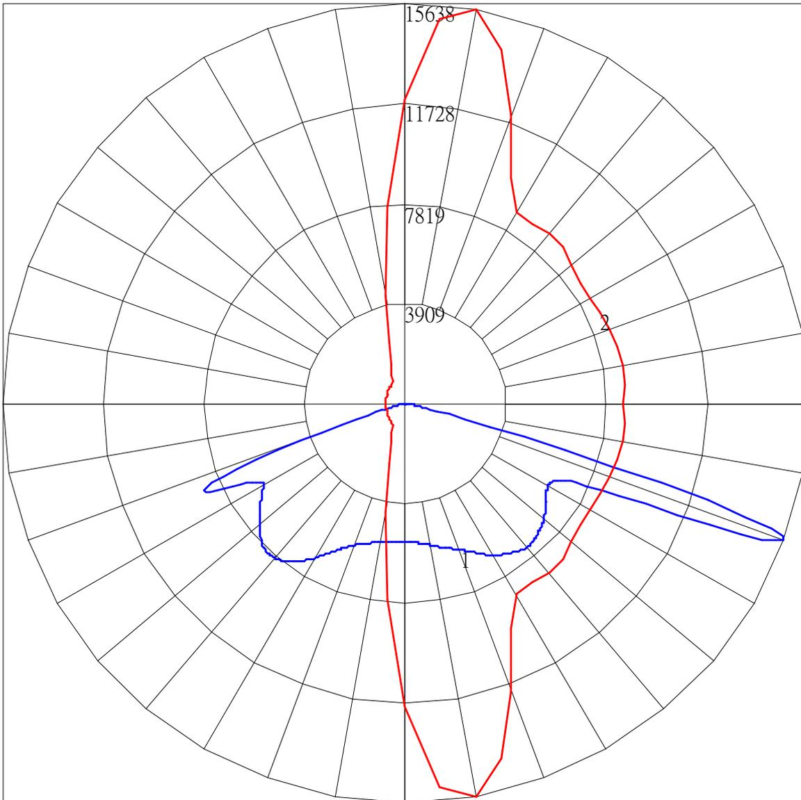
Maximum Candela = 15637.604 Located At Horizontal Angle = 80, Vertical Angle = 70
