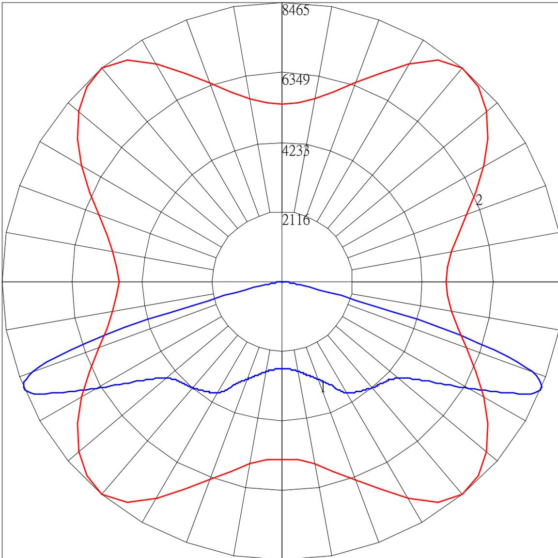
Maximum Candela = 8465.307 Located At Horizontal Angle = 50, Vertical Angle = 67.5
