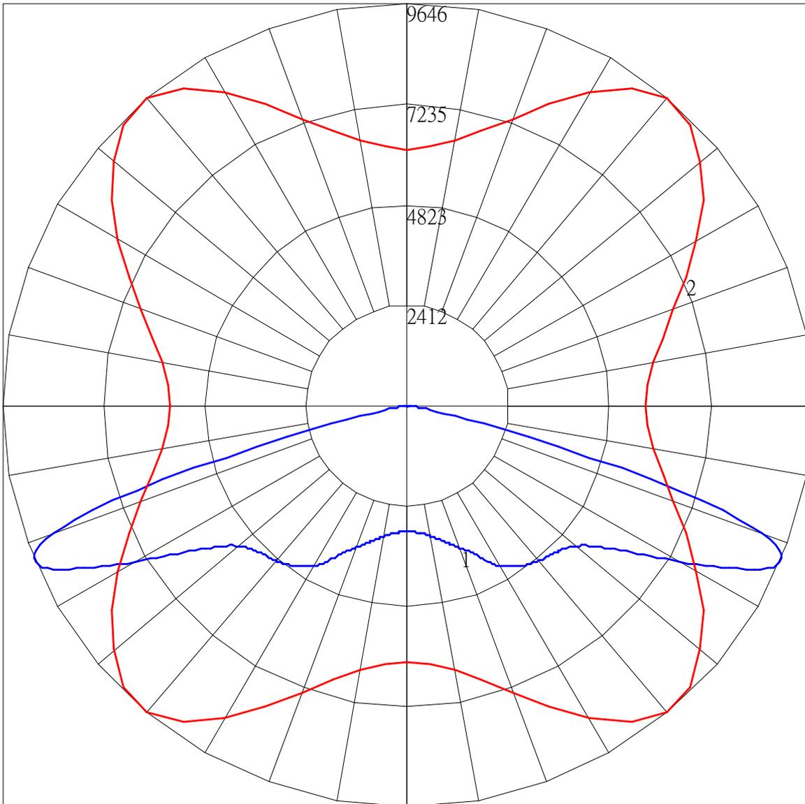
Maximum Candela = 9646.067 Located At Horizontal Angle = 50, Vertical Angle = 67
