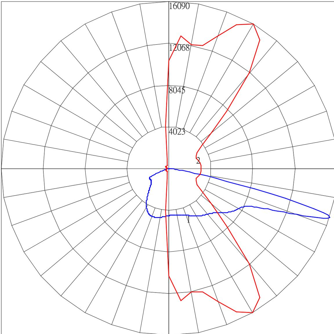
Maximum Candela = 16090.413 Located At Horizontal Angle = 60, Vertical Angle = 73
