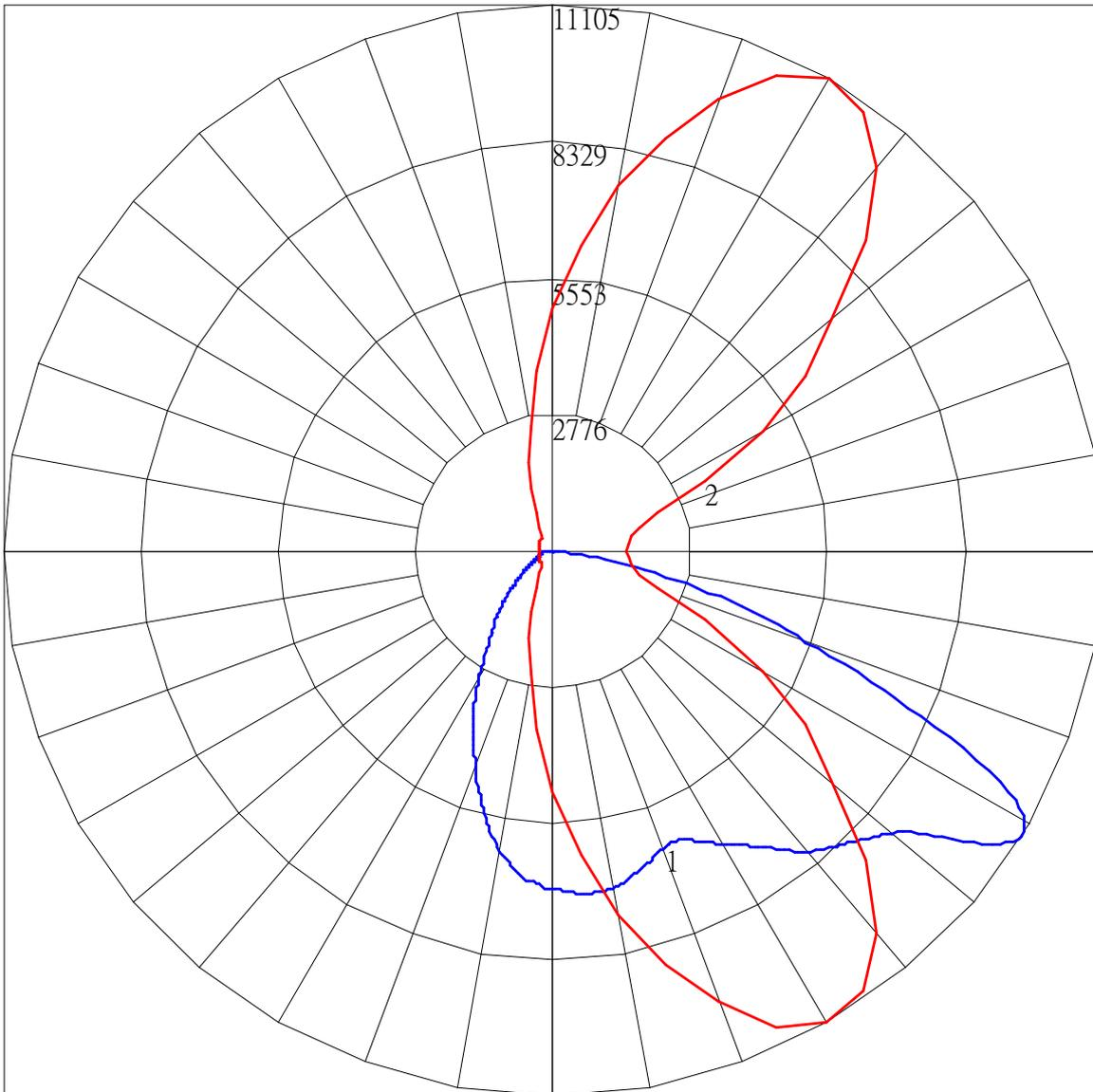
Maximum Candela = 11105.061 Located At Horizontal Angle = 60, Vertical Angle = 58.5
