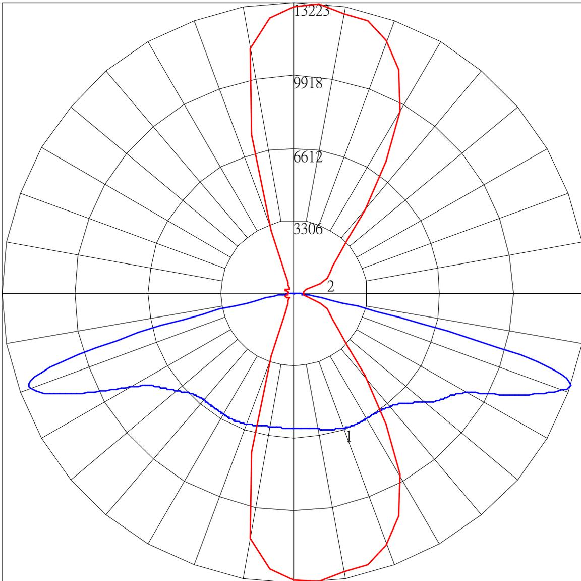
Maximum Candela = 13223.426 Located At Horizontal Angle = 85, Vertical Angle = 71.5
