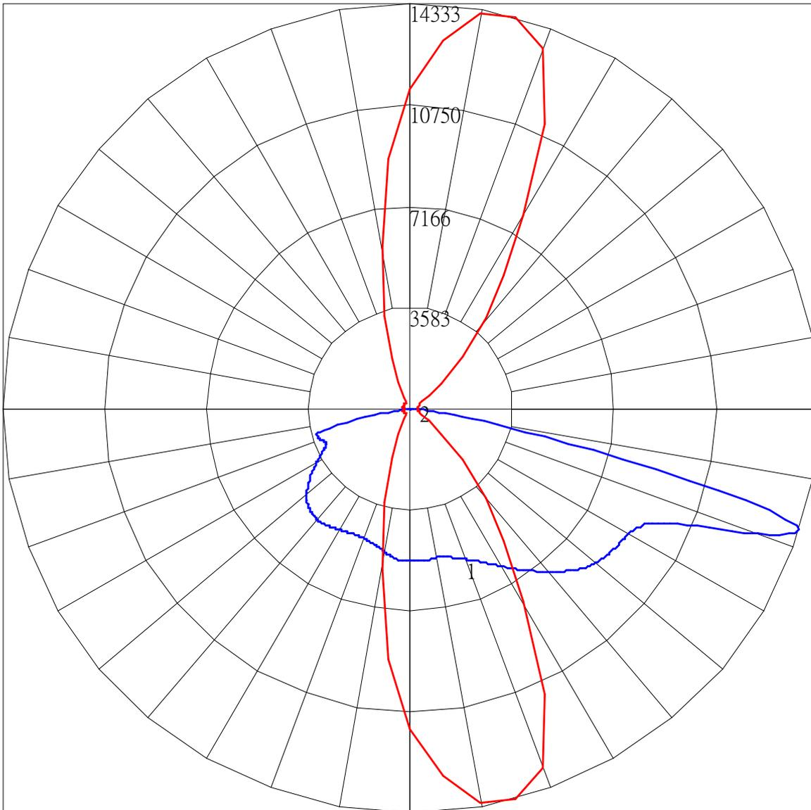
Maximum Candela = 14332.902 Located At Horizontal Angle = 75, Vertical Angle = 72.5
