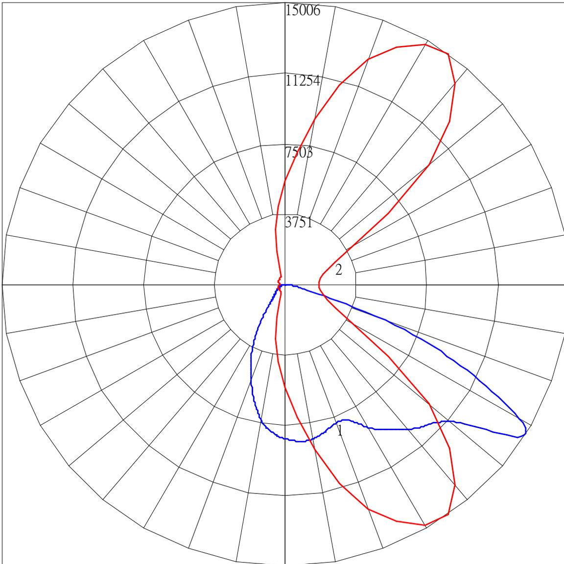
Maximum Candela = 15005.892 Located At Horizontal Angle = 55, Vertical Angle = 58
