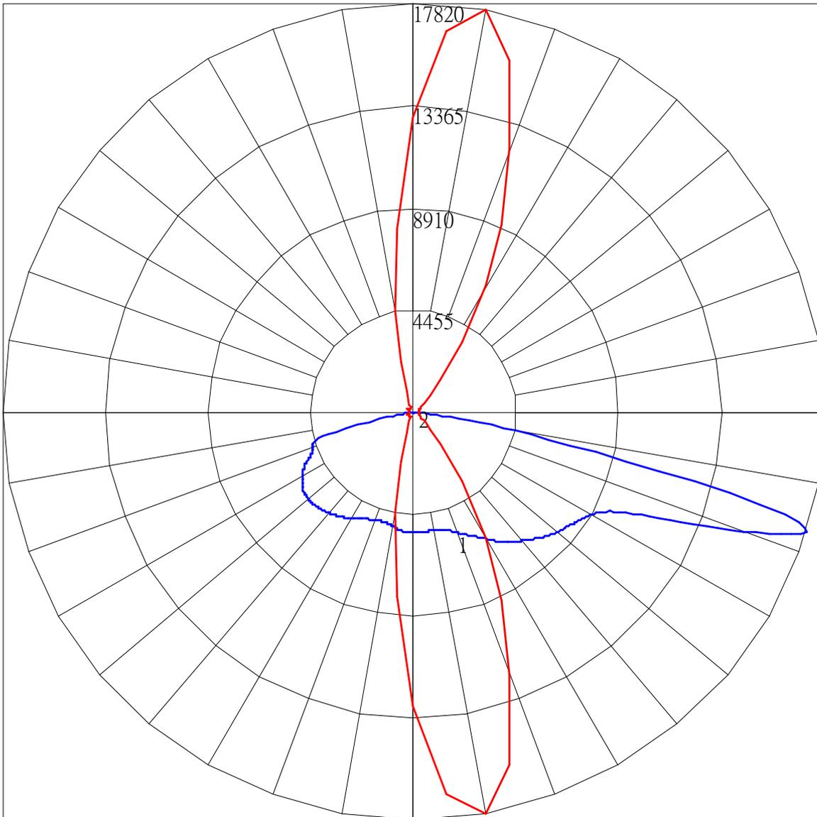
Maximum Candela = 17820.207 Located At Horizontal Angle = 80, Vertical Angle = 73
