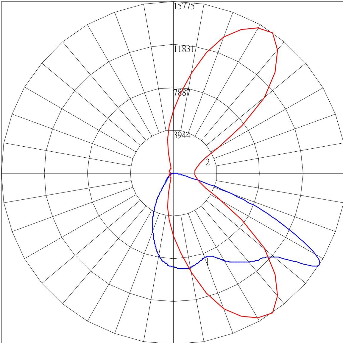
Maximum Candela = 15774.646 Located At Horizontal Angle = 55, Vertical Angle = 57.5
