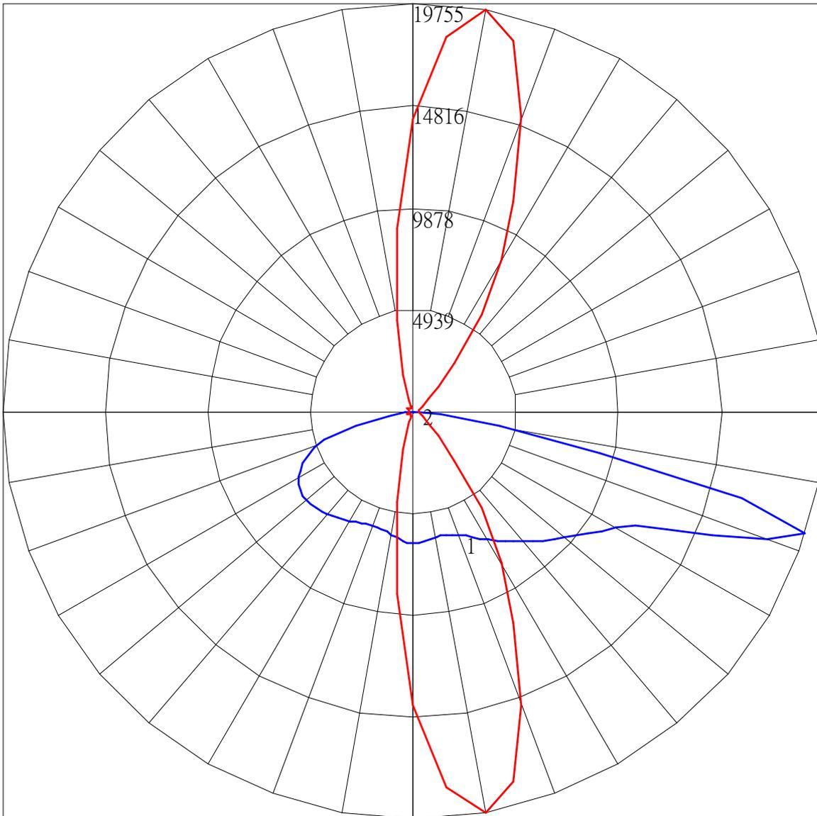
Maximum Candela = 19755.25 Located At Horizontal Angle = 280, Vertical Angle = 72.5
