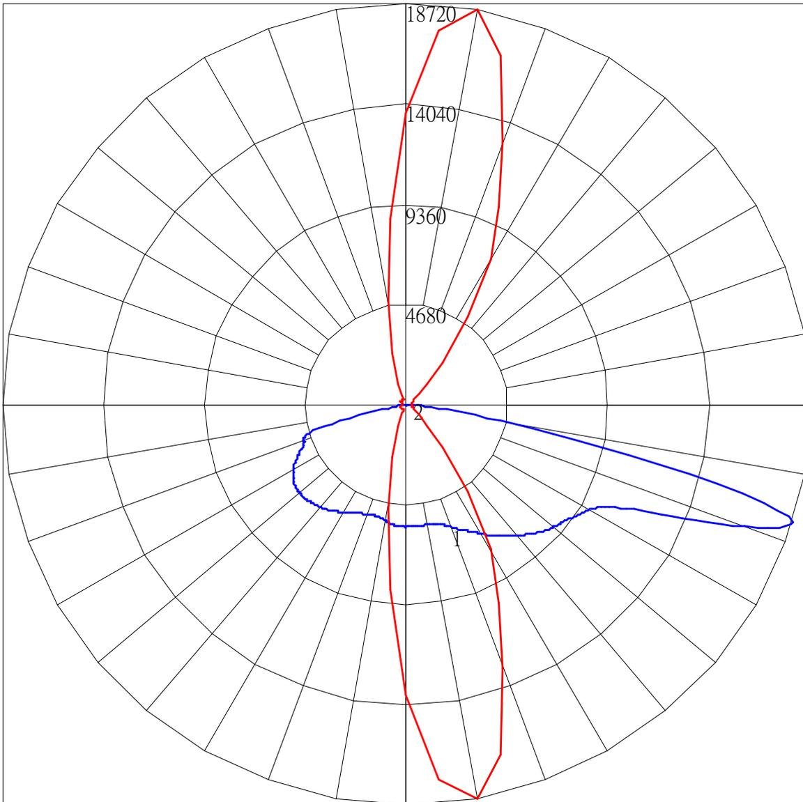
Maximum Candela = 18720.416 Located At Horizontal Angle = 80, Vertical Angle = 72.5
