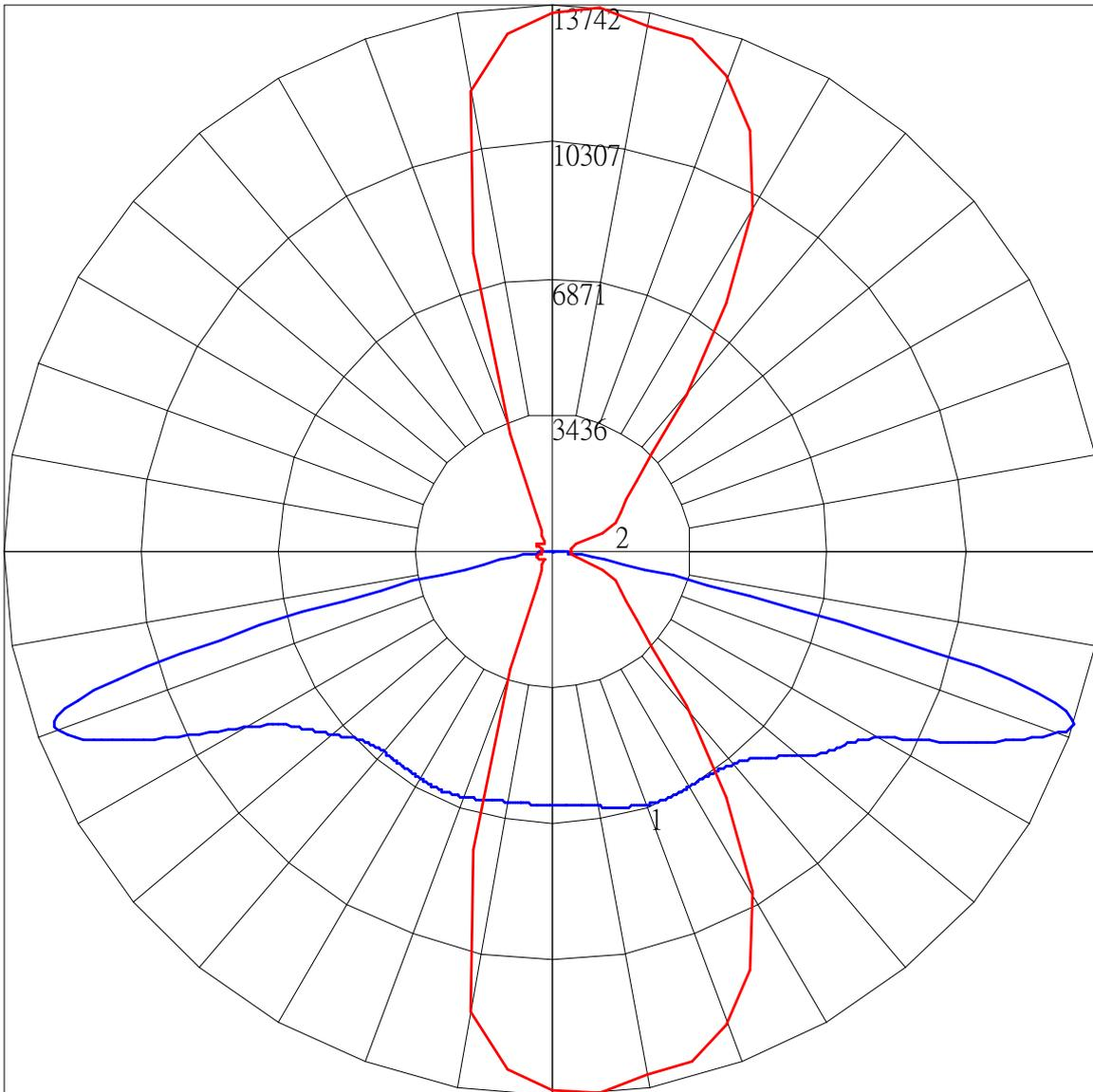
Maximum Candela = 13742.423 Located At Horizontal Angle = 85, Vertical Angle = 71.5
