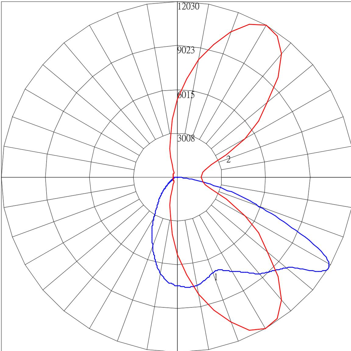
Maximum Candela = 12030.301 Located At Horizontal Angle = 60, Vertical Angle = 58.5
