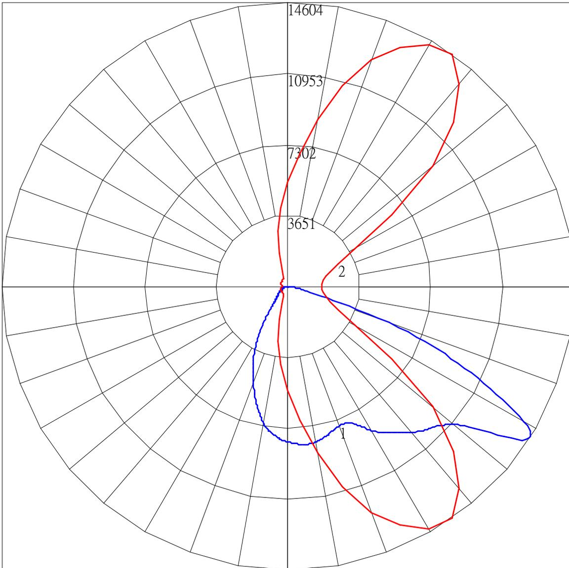
Maximum Candela = 14604.317 Located At Horizontal Angle = 55, Vertical Angle = 58
