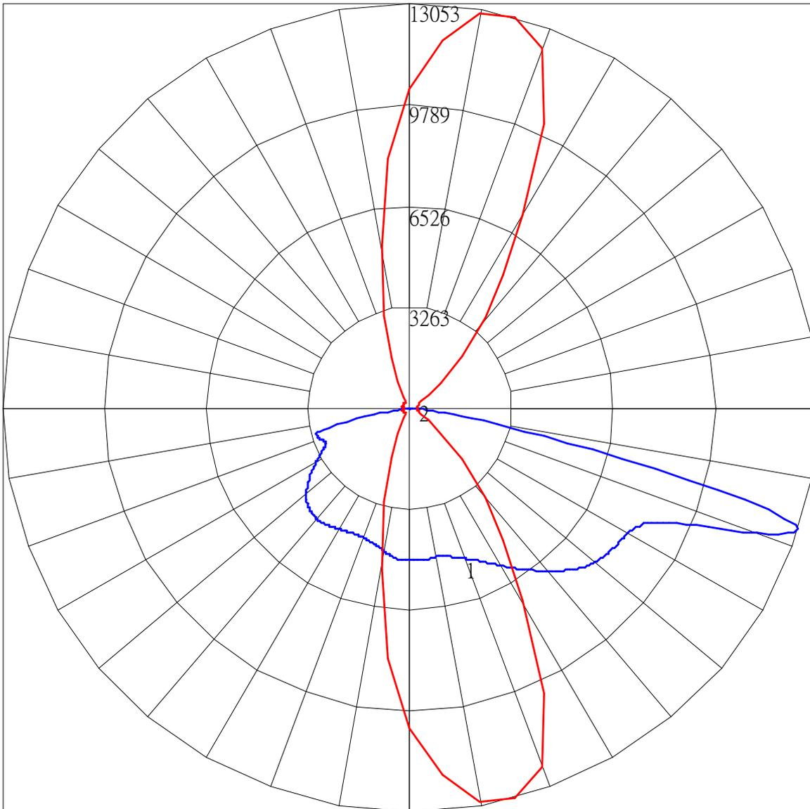
Maximum Candela = 13052.631 Located At Horizontal Angle = 75, Vertical Angle = 72.5
