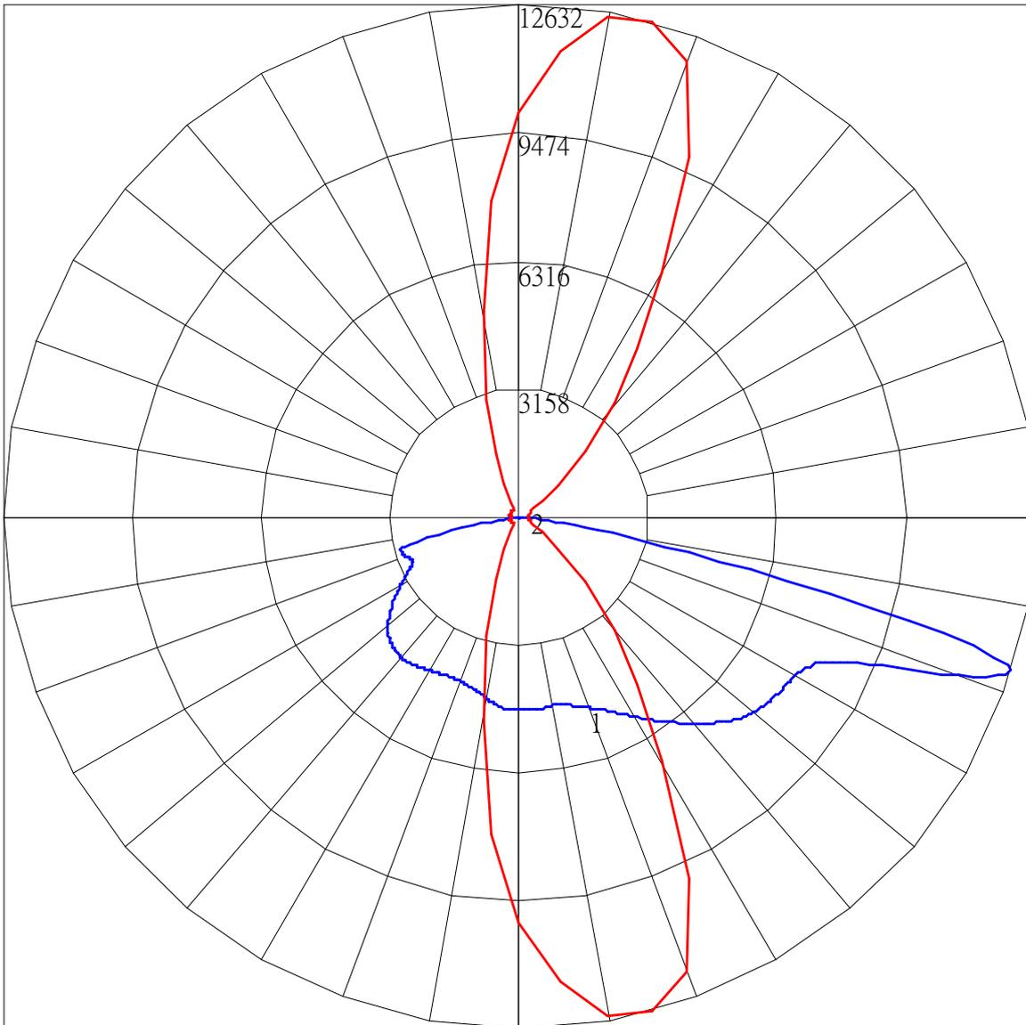
Maximum Candela = 12632.118 Located At Horizontal Angle = 75, Vertical Angle = 72.5
