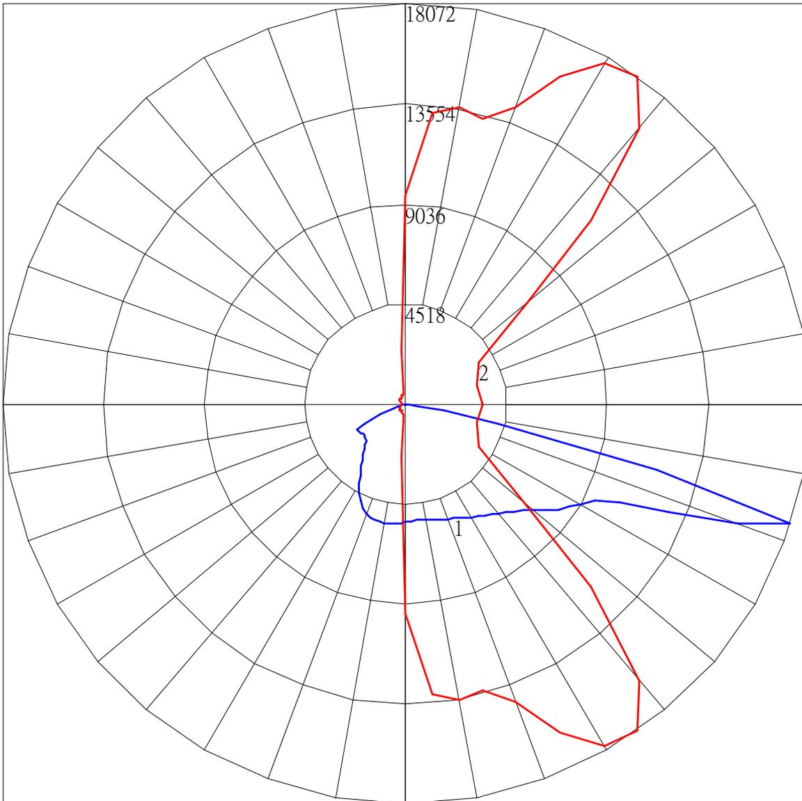
Maximum Candela = 18072.325 Located At Horizontal Angle = 305, Vertical Angle = 72.5
