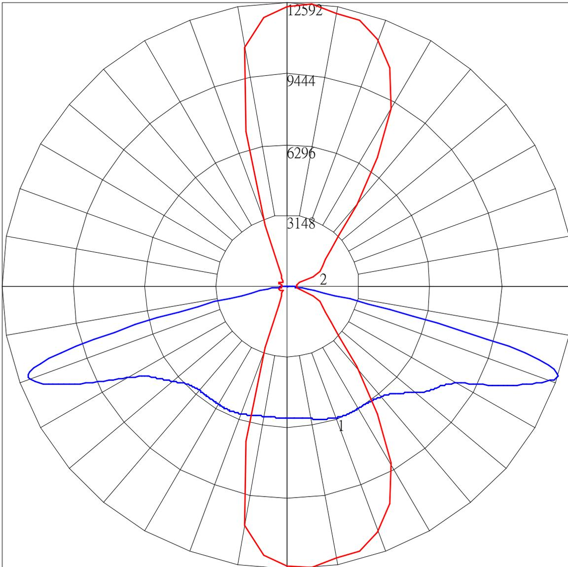
Maximum Candela = 12592.082 Located At Horizontal Angle = 85, Vertical Angle = 71.5
