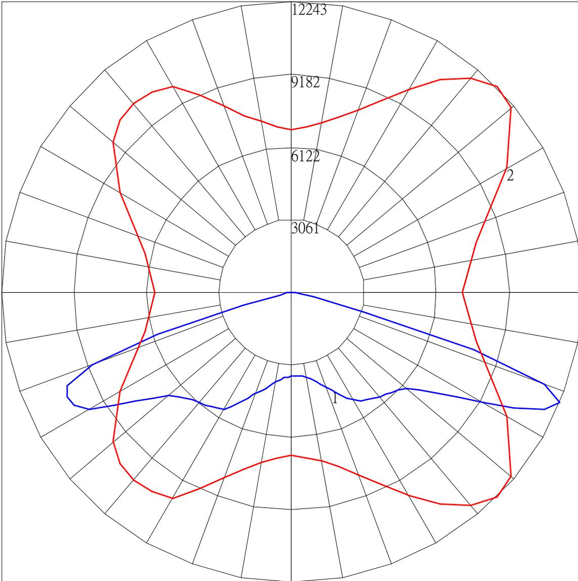
Maximum Candela = 12243.017 Located At Horizontal Angle = 315, Vertical Angle = 67.5
