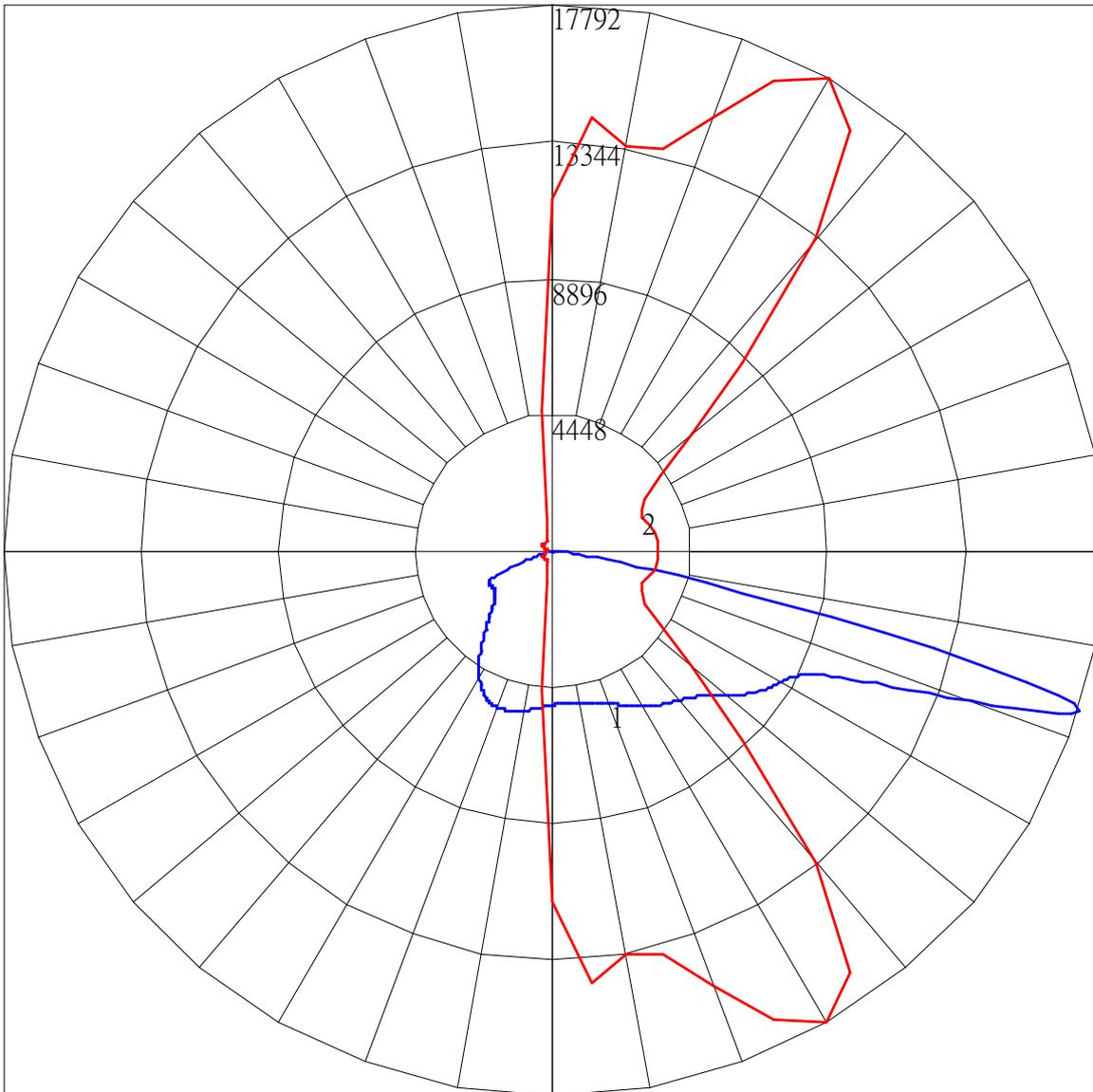
Maximum Candela = 17792.4 Located At Horizontal Angle = 60, Vertical Angle = 73
