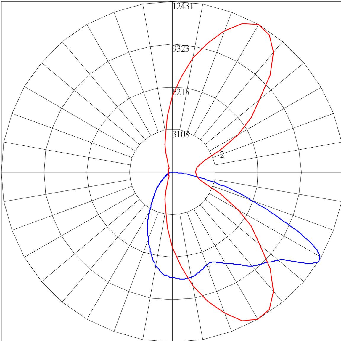
Maximum Candela = 12430.769 Located At Horizontal Angle = 60, Vertical Angle = 58.5
