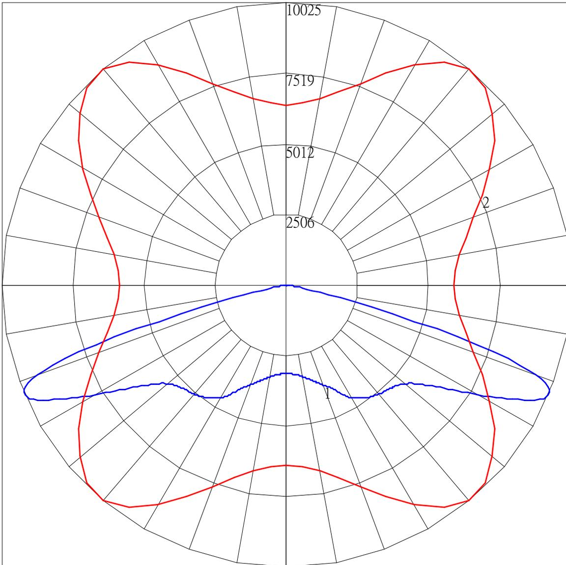
Maximum Candela = 10024.667 Located At Horizontal Angle = 50, Vertical Angle = 67
