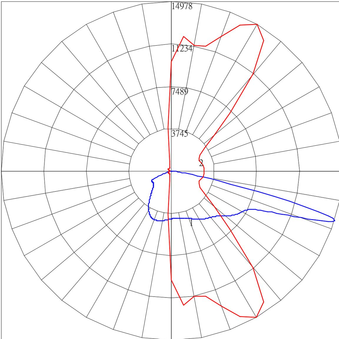
Maximum Candela = 14978.392 Located At Horizontal Angle = 60, Vertical Angle = 73
