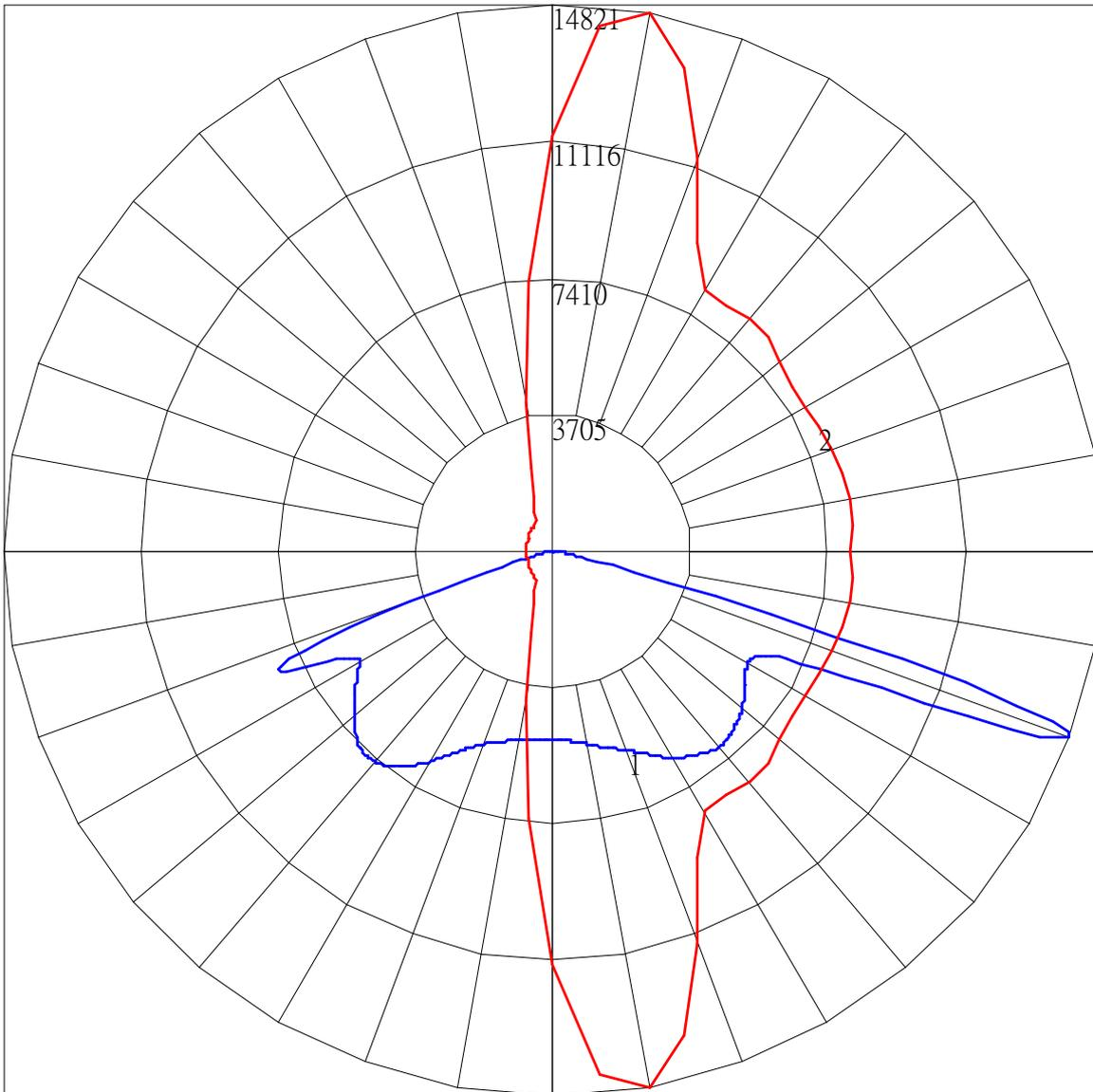
Maximum Candela = 14820.774 Located At Horizontal Angle = 80, Vertical Angle = 70
