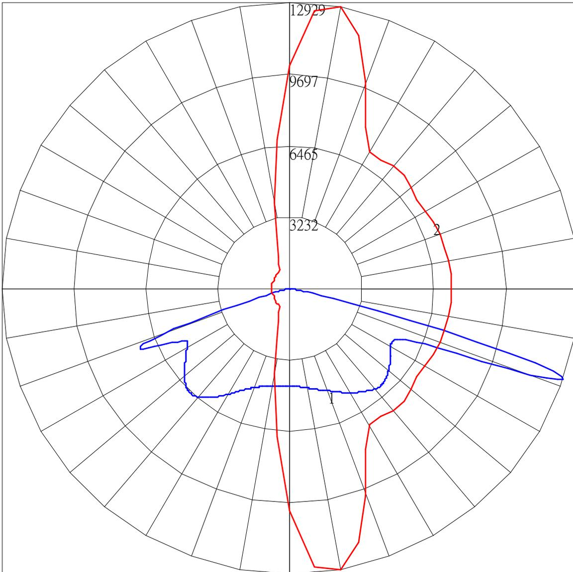
Maximum Candela = 12929.242 Located At Horizontal Angle = 80, Vertical Angle = 71.5
