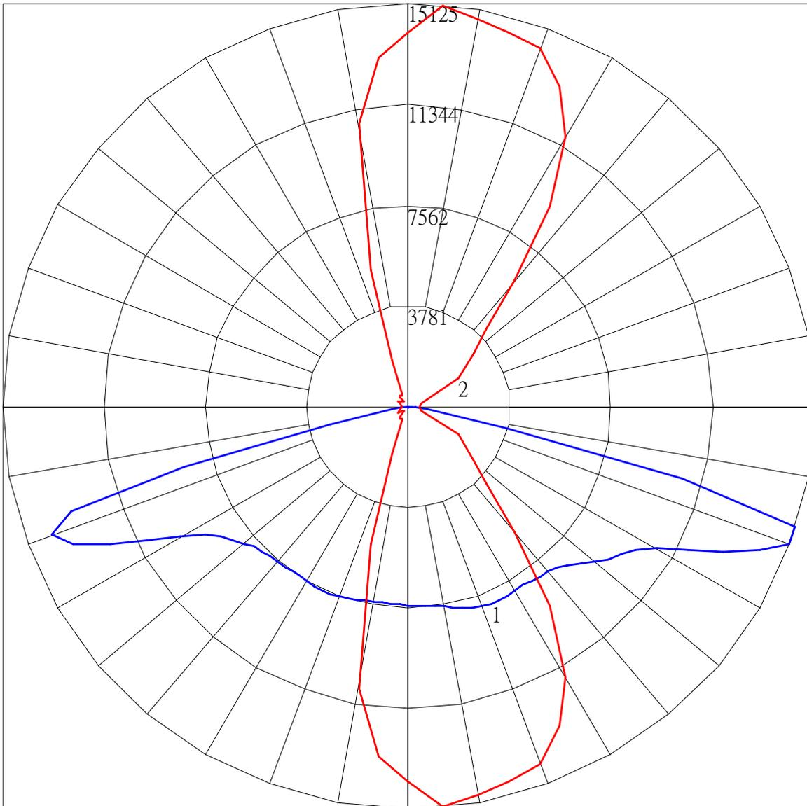
Maximum Candela = 15124.693 Located At Horizontal Angle = 275, Vertical Angle = 72.5
