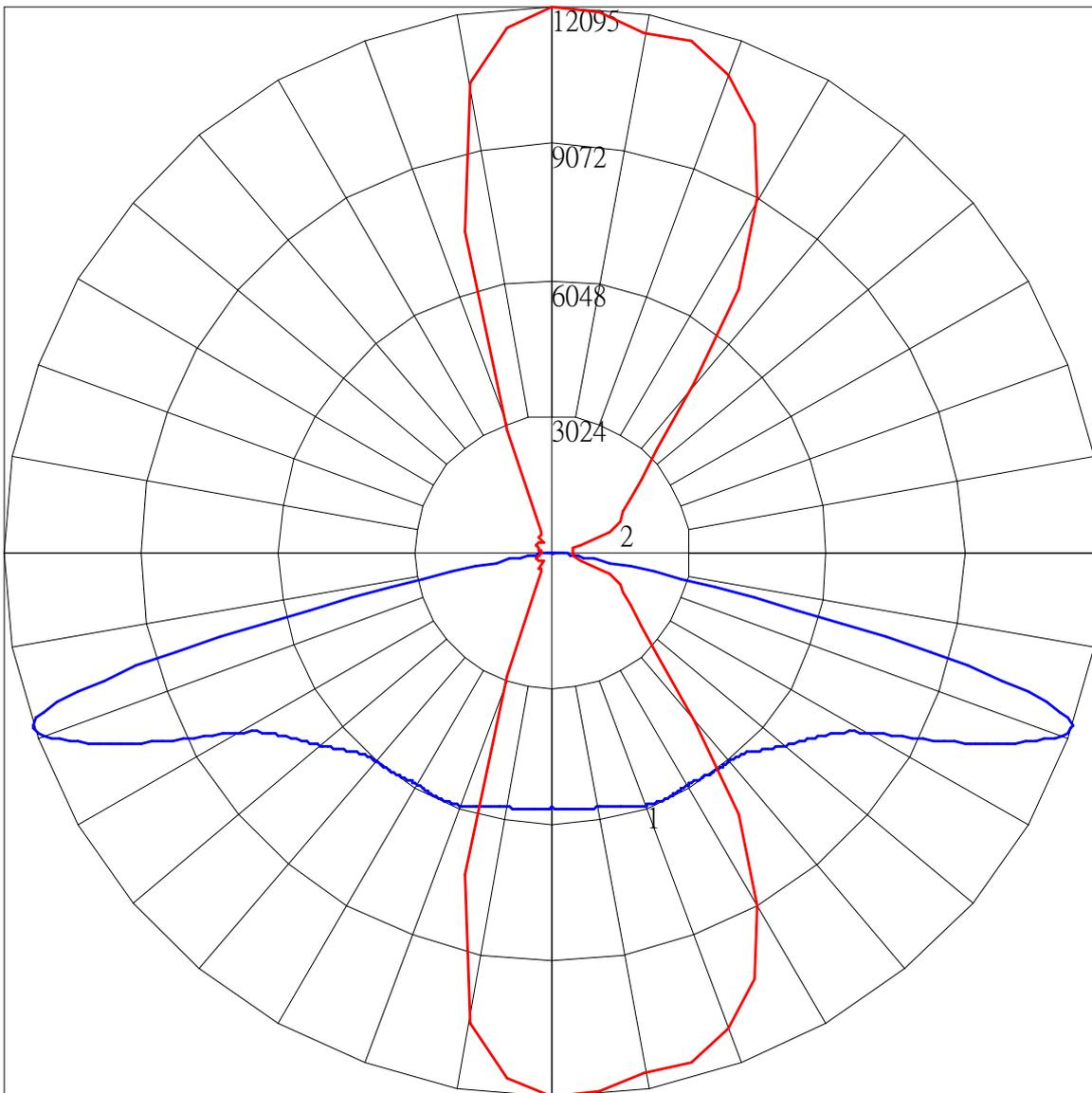
Maximum Candela = 12095.418 Located At Horizontal Angle = 90, Vertical Angle = 71
